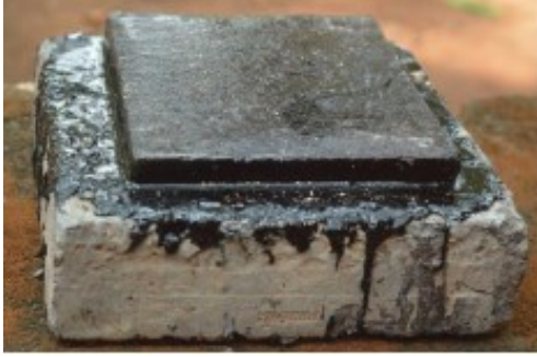
Figure X Bitumen used to adhere coir pith tiles on concrete
