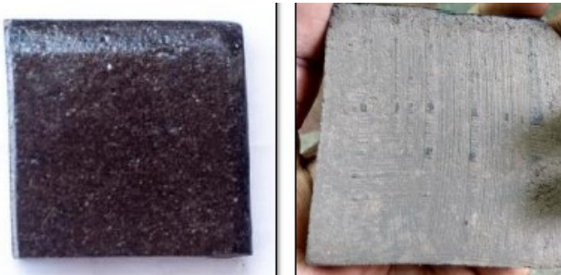
Figure IX Sample before and after Abrasion test
